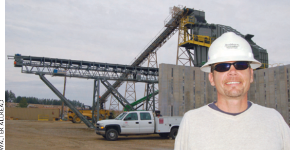
Buckhorn General Manager Rich Moses says rocks are hauled from the quarry pit, right, dumped in the primary crusher then conveyed to a secondary crushing and screening tower behind him to be sized.
